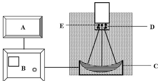
Figure 2. Experimental setup with a schematic diagram of the high-frequency HIFU apparatus: arbitrary waveform generator (A), radio-frequency power amplifier (B), acoustic lens transducer (C), water bath (D), and polymer micelles (E).
