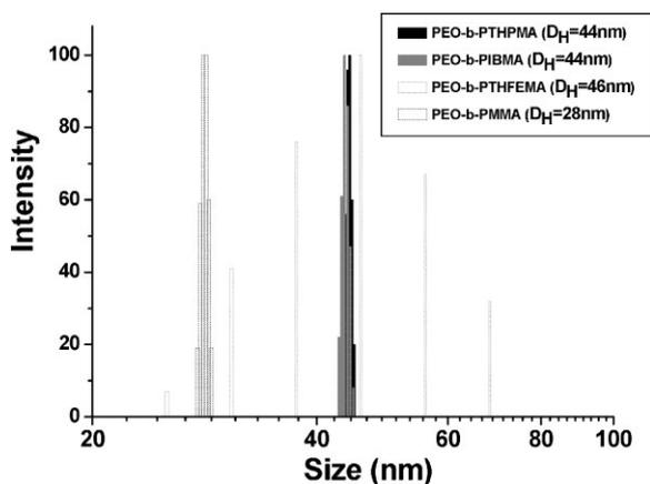
Figure 3. Size distributions of different BCP micelles in aqueous solution as revealed by DLS (the average hydrodynamic diameters are indicated in the figure).
