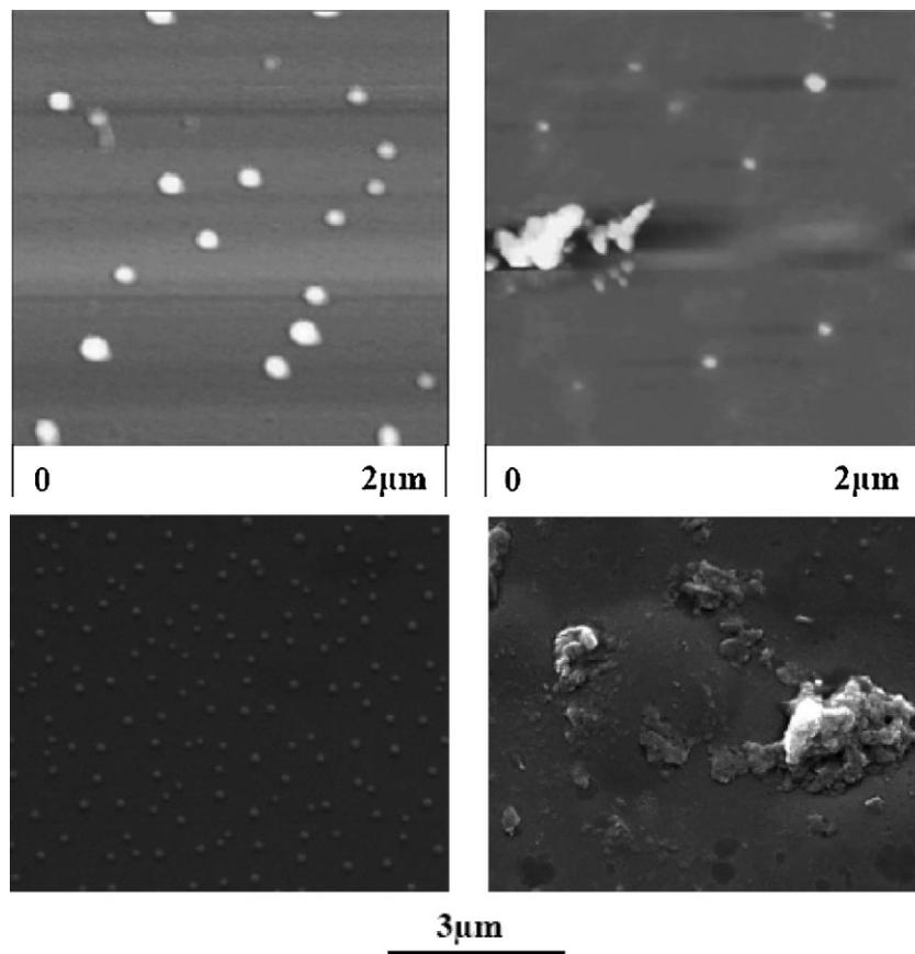
**Figure 8.** Images of AFM (upper) and SEM (lower) showing micelles of PEO-*b*-PIBMA before ultrasound (left) and large aggregates formed from disrupted micelles after ultrasound irradiation (right).
