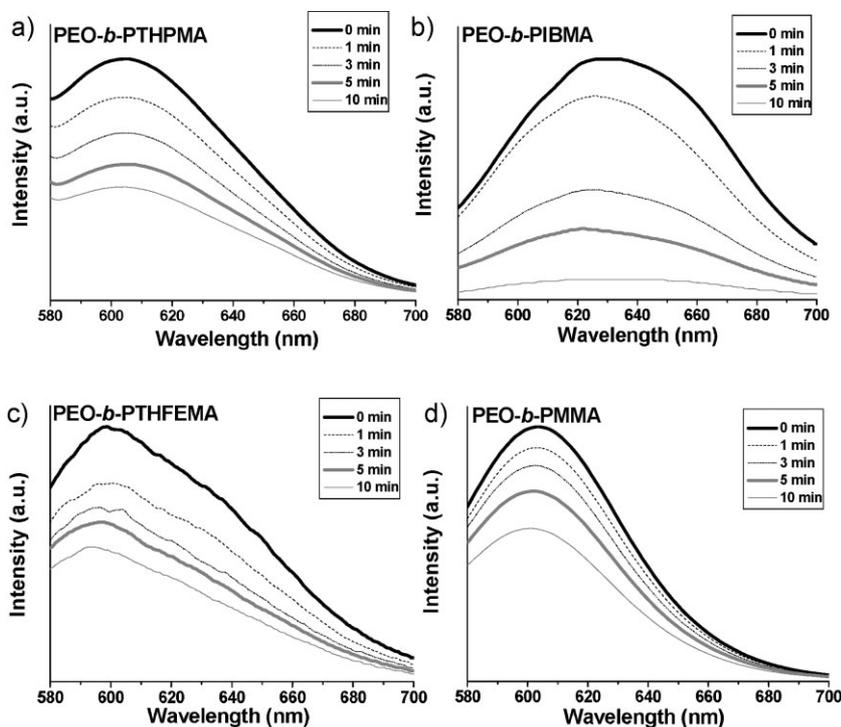
**Figure 5.** Fluorescence emission spectra of NR-loaded BCP micelles (excitation: 540 nm) recorded at different ultrasound irradiation times for (a) PEO-*b*-PHTPMA, (b) PEO-*b*-PIBMA, (c) PEO-*b*-PTHFEMA, and (d) PEO-*b*-PMMA, all experiments being carried out under the same conditions (ultrasound power: 40 W, micellar solution volume: 5 mL).
