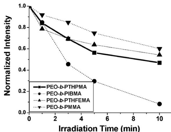
**Figure 6.** Normalized fluorescence emission intensity of NR versus ultrasound irradiation time for various BCP micellar solutions, using data in Figure 5 with the intensity measured at the respective emission maximum of each BCP.
