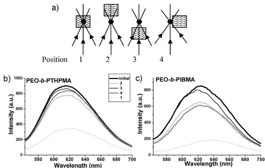
Figure 10. (a) Schematic of different positions of the focal spot of ultrasound beams with respect to micellar solution. (b) and (c) Fluorescence emission spectra of NR (excitation 540 nm) recorded after 5 min ultrasound irradiation (40 W) with different focal spot positions for micelles of PEO-b-PTHMPMA (b) and PEO-b-PIBMA (c).
