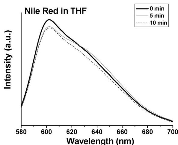
Figure 4. Fluorescence emission spectra of NR dissolved in THF (excitation: 540 nm) recorded before (0 min) and after exposure to ultrasound irradiation (5 and 10 min) (ultrasound power: 40 W, solution volume: 5 mL).
