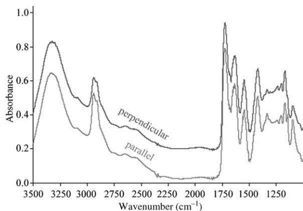
Figure 3. Polarized infrared spectra at room temperature for a film of peptide/PVA (24 wt %) stretched to 100% strain at 95°C.
