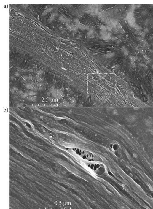
Figure 5. SEM images for films of peptide/PVA (24 wt%) on a silicon wafer cast from a  $0.5 \text{ mg mL}^{-1}$  solution of the complex. Image b shows the magnification of the marked region on image a.
