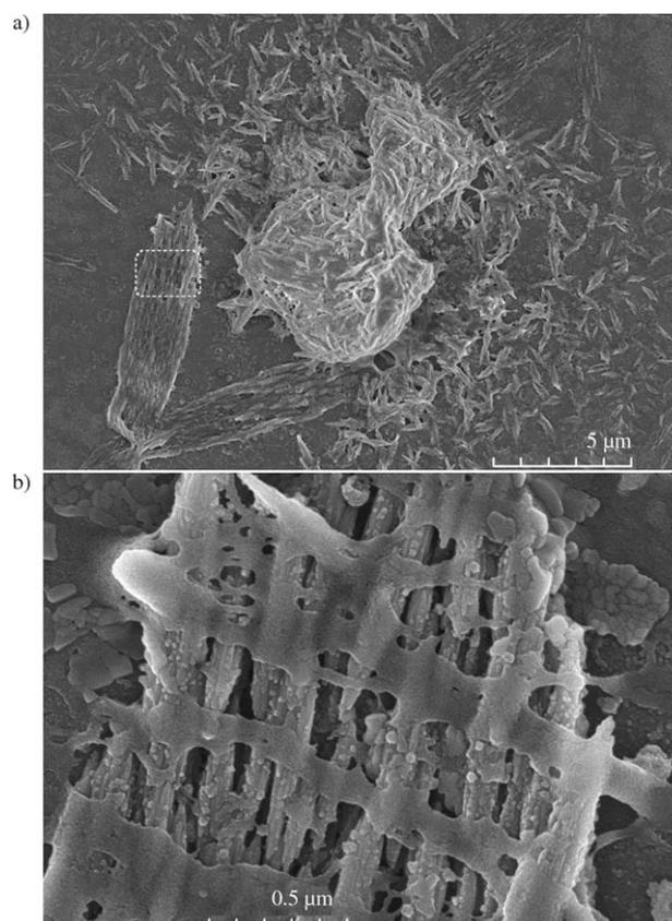
Figure 4. SEM images for films of peptide/PVA (24 wt %) on a silicon wafer cast from a 0.1  $\text{mg mL}^{-1}$  solution of the complex. Image b shows the magnification of the marked region on image a.
