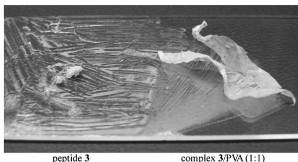
Figure 2. Photo showing **3** in an oily state at room temperature and the peelable film of the peptide complexed with 9.4 wt % PVA.
