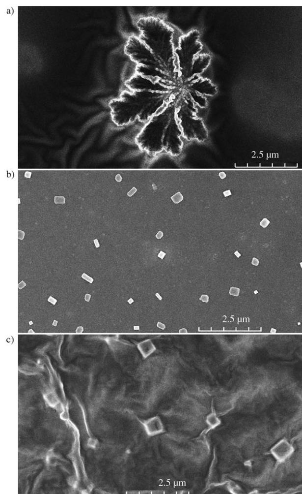
Figure 6. SEM images for a) pure functionalized peptide **3**, b) pure unfunctionalized peptide **1**, and c) unfunctionalized peptide **1** blended with 90 wt % of PVA.
